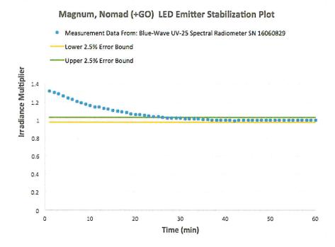
Measurement data for 60 minutes (maintains this level indefinitely over time). The stabilization time from the above data is 30 minutes.
