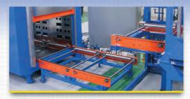
An integrated conveyor elevator raises and advances nested parts to the first dip station. The lowerator automatically returns to the conveyor level to receive the next batch of parts.
