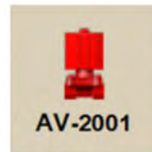
Figure 1-4, NC Shutoff Valve Faulted
