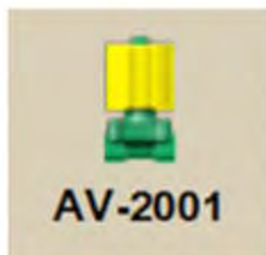
Figure 1-2, NC Shutoff Valve in Manual On Mode
