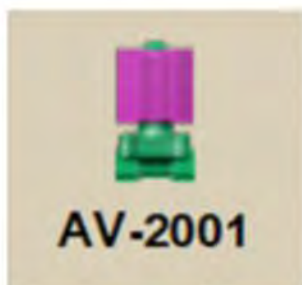
Figure 1-1, NC Shutoff Valve in Auto On Mode
