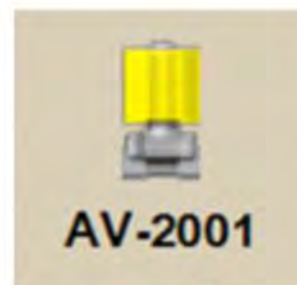
Figure 1-3, NC Shutoff Valve in Manual Off Mode
