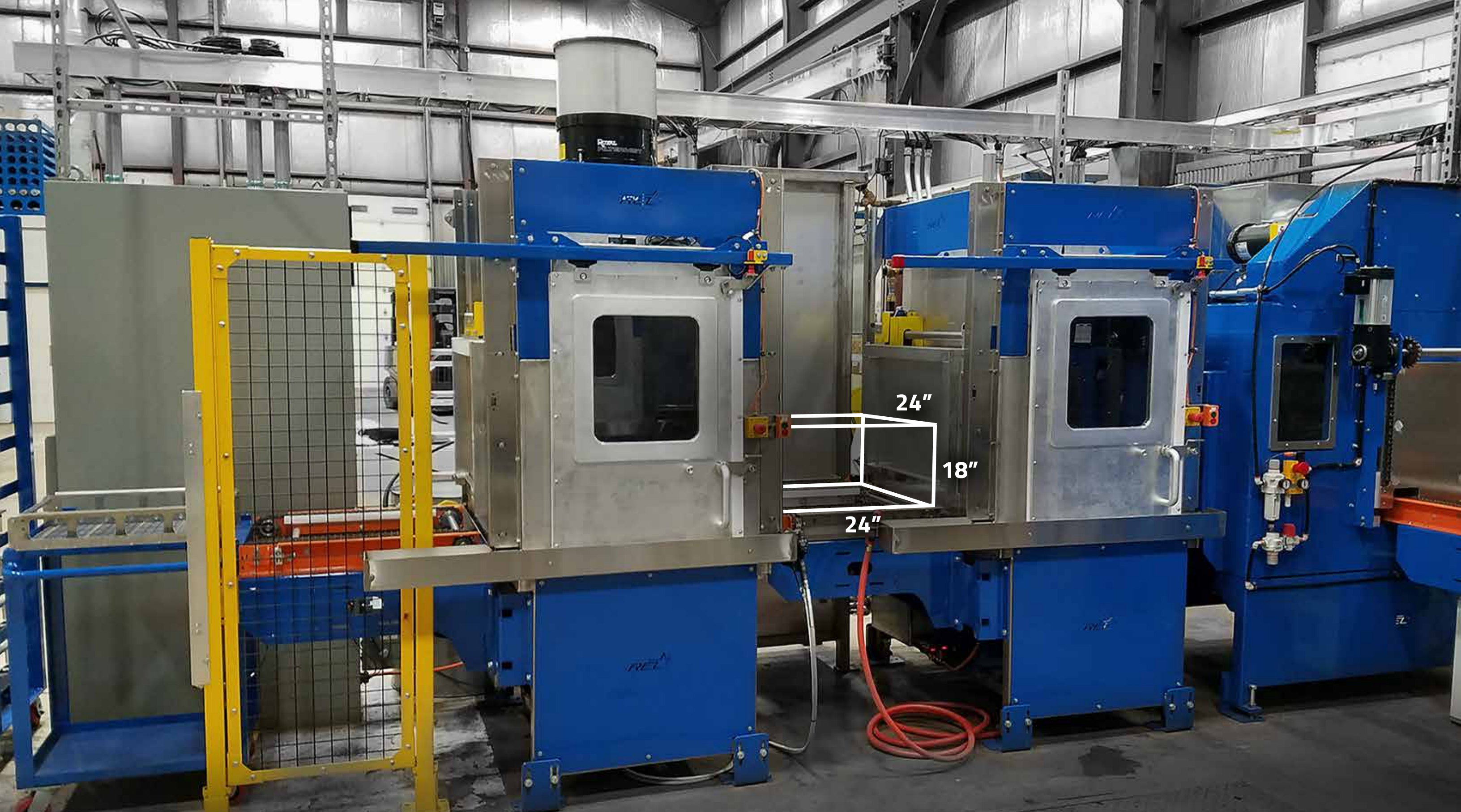
Fluorescent Penetrant Inspection Line Model #RCF242418
